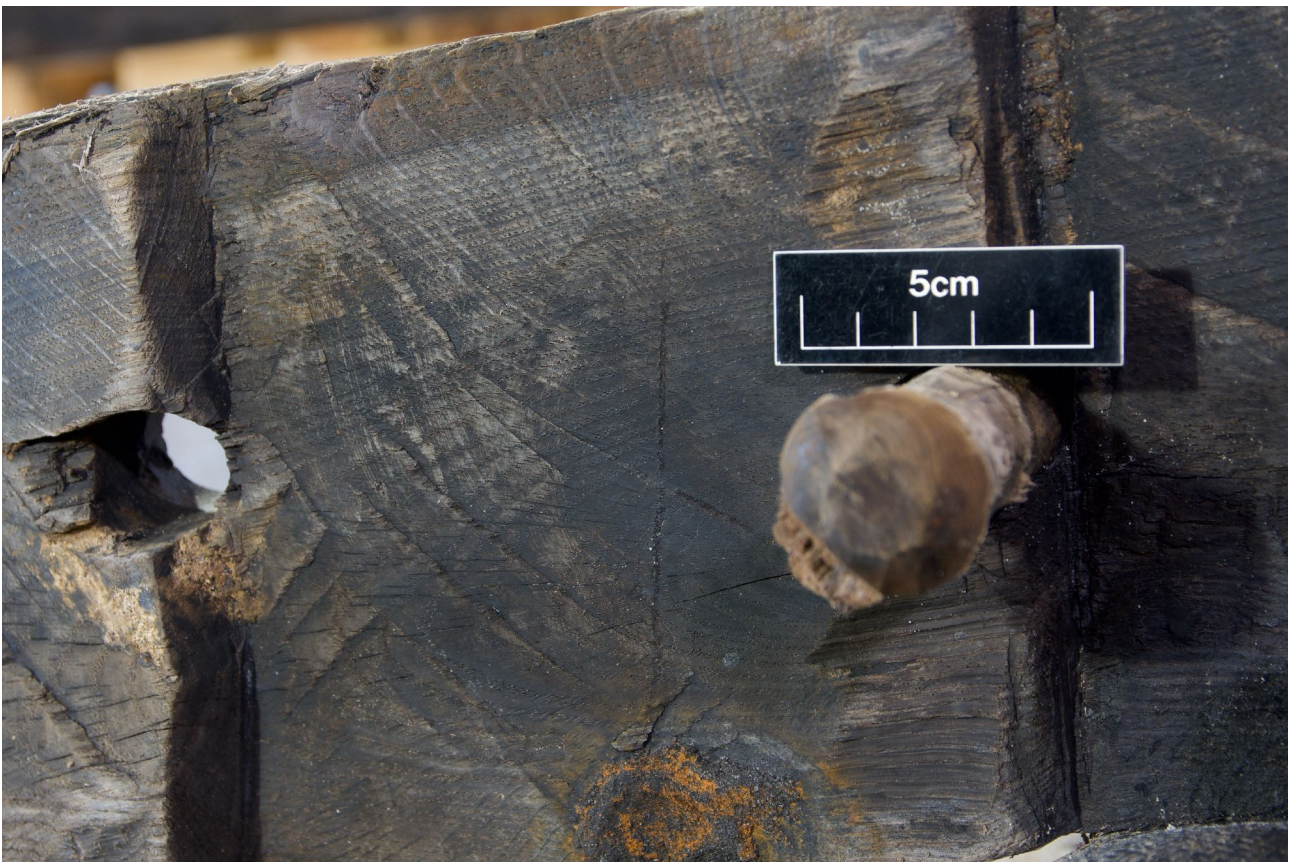
Detail shot of axe marks in the joggle of a clinker frame.
